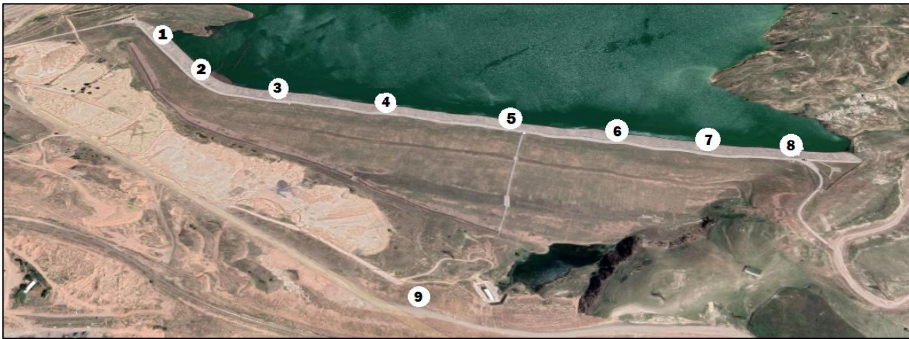
Figure 2. Microseismic measurement points along the Ohangaron Reservoir dam
