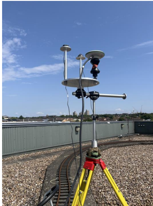
Fig. 4: Rooftop test configuration used for the quasi-static experiment at the NGI, including a Leica 360 prism, a Leica AS10 geodetic antenna connected to both Leica GS10 and u-blox F9P receivers, and Tallysman TWI 3972 and patch antennas paired with separate u-blox F9P receivers.
