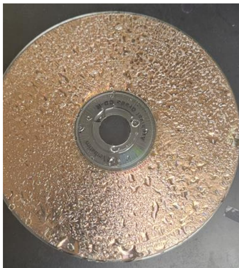
149 Supplementary Figure 20. CD after the nitric acid soak.
