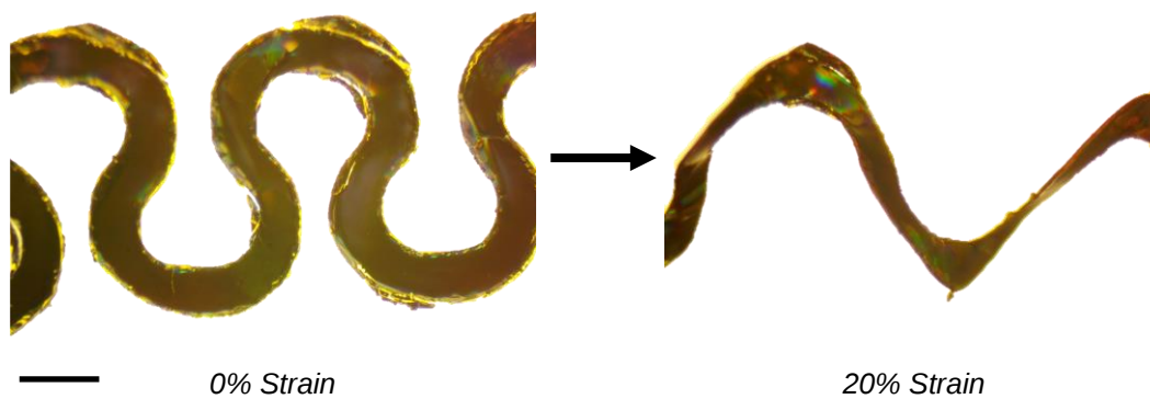
92 Supplementary Figure 2. Photograph of the UCDEs during stretching (scale bar 1 mm).
