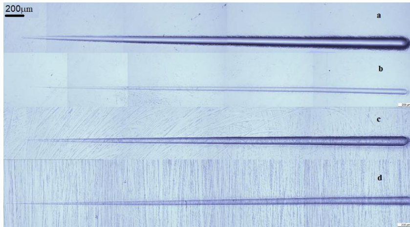
Representative optical micrographs of scratch tracks produced on AISI 420 MOD steel under different substrate conditions: (a) untreated, (b) quenched, (c) Tenifer-treated, and (d) quenched plus Tenifer-treated.
