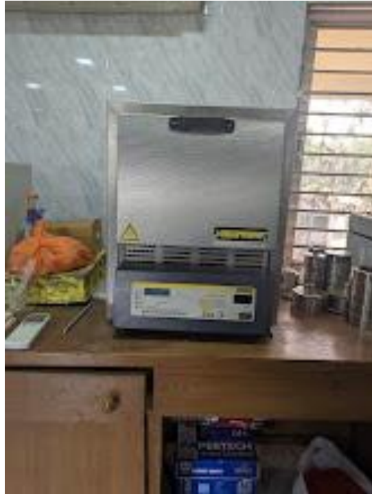
Figure 5. Vacuum furnace (Shanghai Chen Hua Electric Furnace Corp.) used for sintering at 1100 °C.
