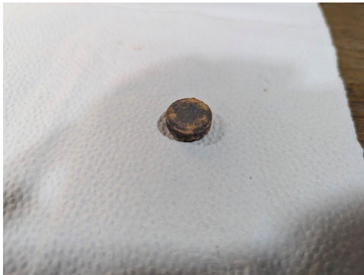
Figure 6. Sintered Ti/SiO 2 composite pellet after vacuum sintering, showing brownish-grey surface which intended surface oxidation and good consolidation.
