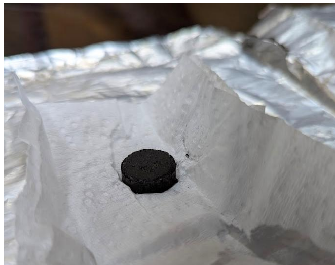
Figure 4. The cylindrical disc geometry ( \sim 10 mm diameter \times 5 mm height) was created by applying green compact after 200 MPa compaction prior to sintering.
