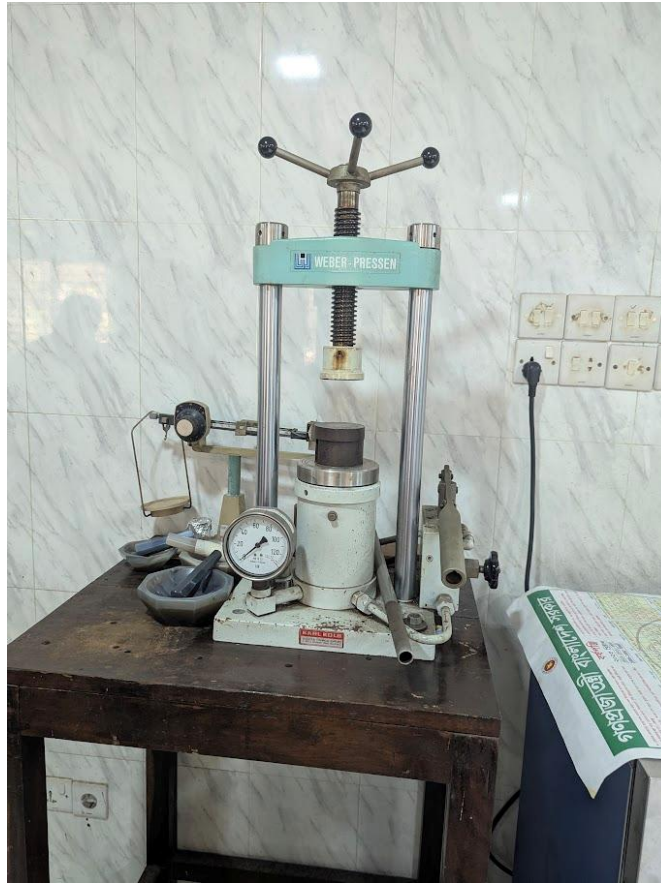
Figure 3. 200 MPa uniaxial compaction performed with Weber-Pressen hydraulic press.
