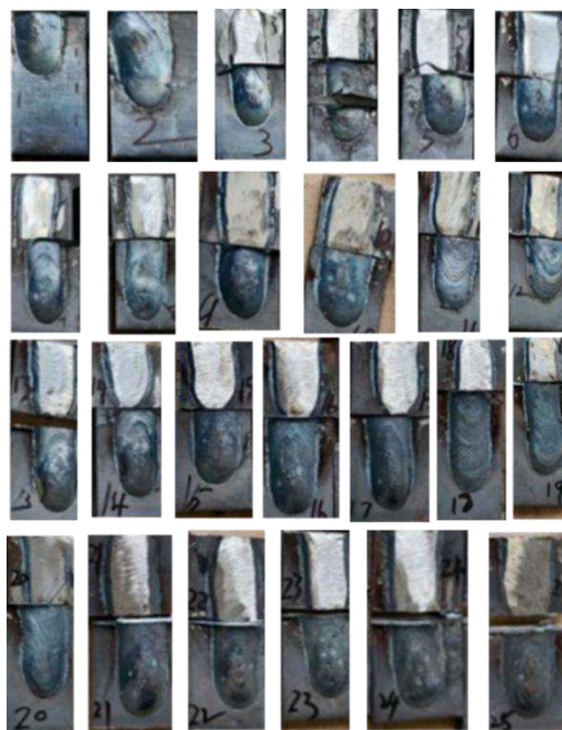
Fig. 3 25 sets of formulas corresponding to the appearance of weld seams
