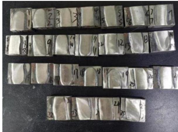
Fig. 9 Processing sample diagram for testing the composition content of weld seam components
