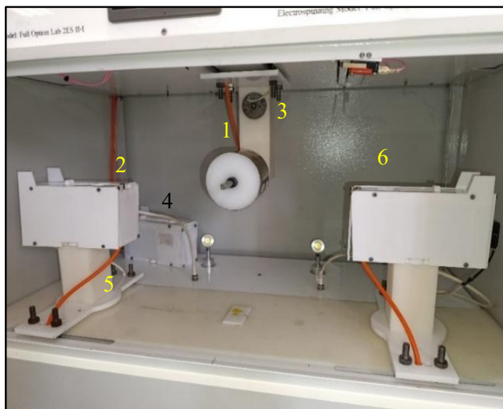
Figure 1. The electrospinning apparatus components [1: rotating plate, 2: Injector, 3: adjustable rotating plate, 4: magnetic field, 5: holder, 6: fiber container].
