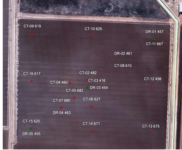
Fig. 1: The 16 sensors are distributed across 64 hectares ( 800m \times 800m ) labelled CT-X YYY, where X ranges from 01 – 16. These are subsequently referred to as ct_X in analyses. The sensors provide full coverage of the farm, with greater concentration towards the centre, where the weather station is located. The sensors designated as DR-X are soil moisture measurement devices and are excluded from the present analysis. The furrow irrigation occurred from the east (right) and travelled across the farm.
