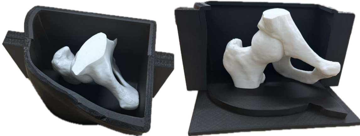
Figure 1 3D Printed Surface Mold with Hip & Femur
