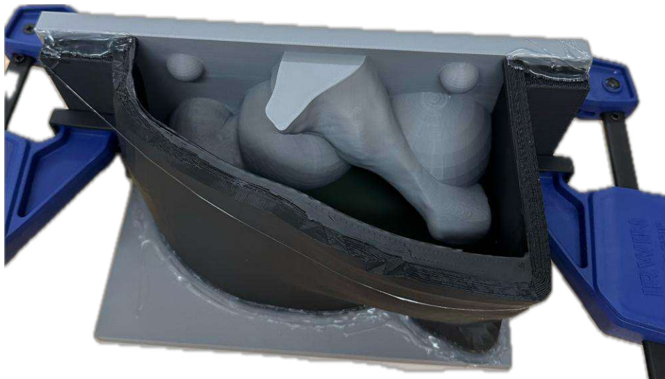
Figure 123 Pouring Ballistics Gel Into Front Mold
