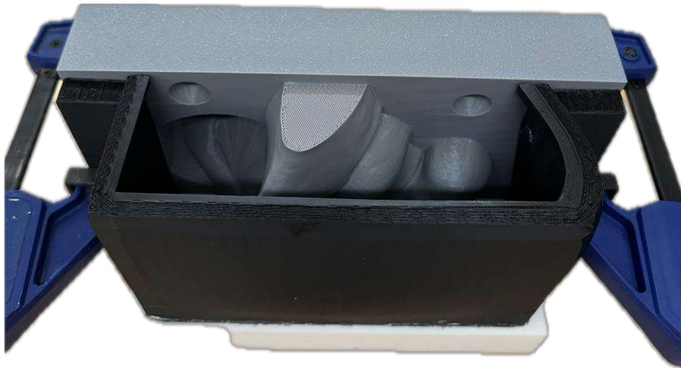
Figure 122 Pouring Ballistics Gel Into Back Mold
