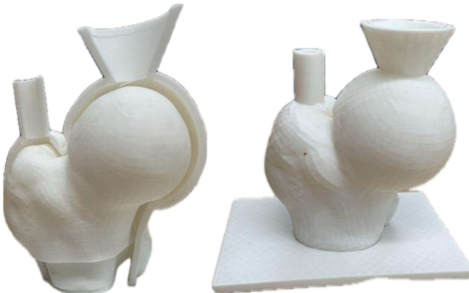
Figure 2 3D Printed Joint Capsule Mold
