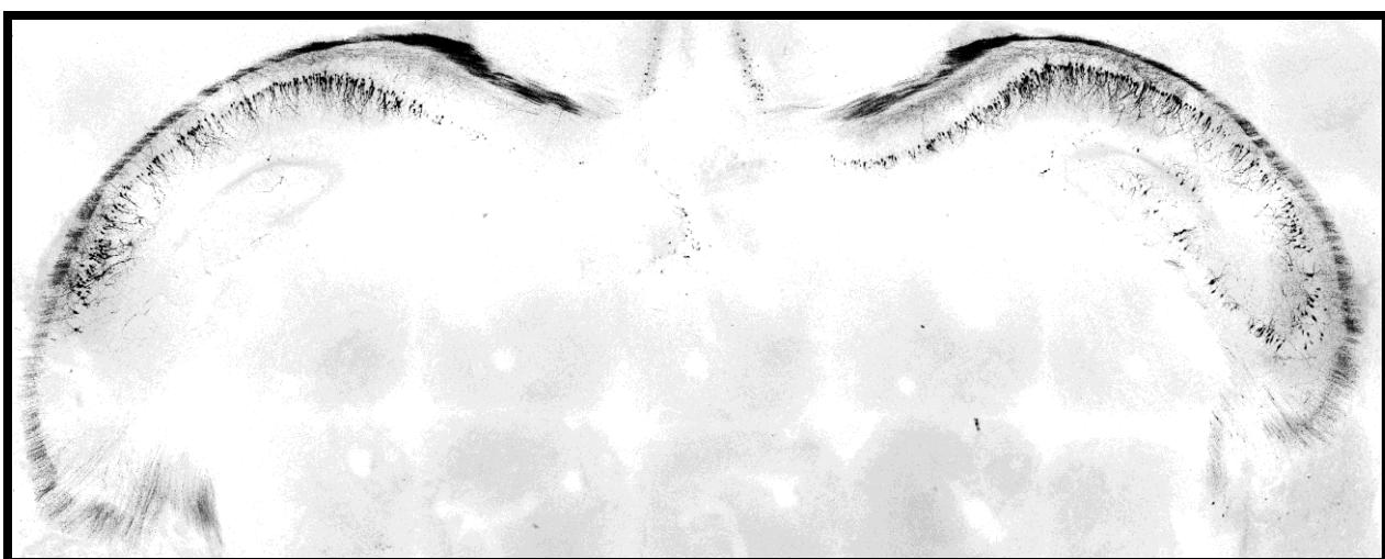
Confocal image example of bilateral transfection of EGFP in rat hippocampus with the usage of the tripolar electrode configuration. Black cells are neurons expressing GFP.
